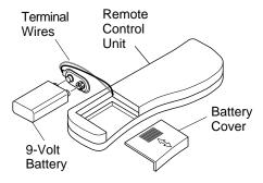
Figure 32 - Installing Battery in Hand-Held Remote Control Unit (CGHRCTA Series)
